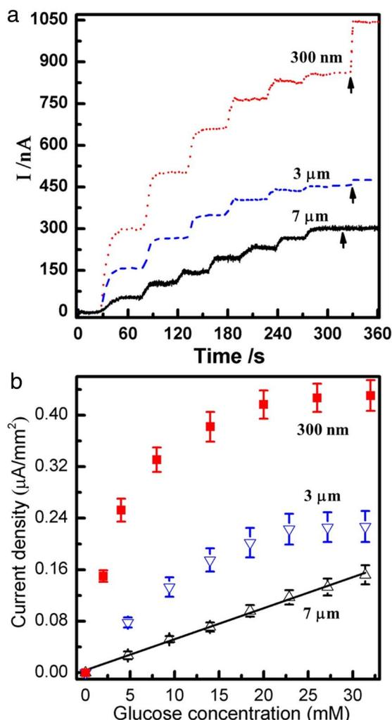
**Figure 6.** (a) Chronoamperometry of glucose sensor response to glucose concentration with printed GOx on Pt working electrodes and 300 nm, 3 μm and 7 μm thick outer PFSA membrane. Arrows indicate addition of 0.13 mM acetaminophen. (b) Current density vs. glucose concentration for these devices.
