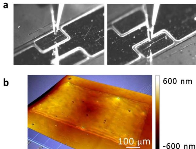
**Figure 5.** (a) E-jet printing of enzyme ink on Pt working electrodes of glucose sensor and (b) optical profilometry images of  $400 \times 800$  μm<sup>2</sup> (working electrode size) pad printed twice over the same area at  $f = 20$  Hz,  $v = 500$  μm/s.
