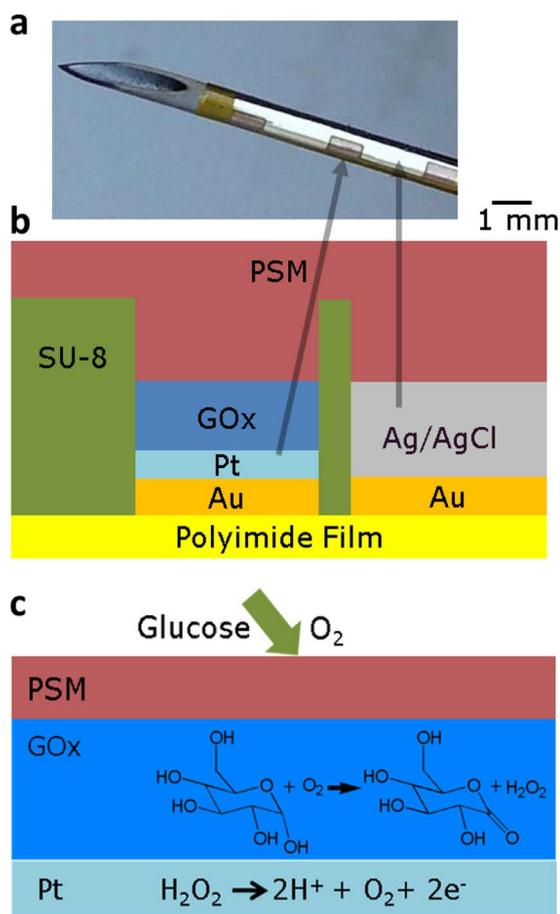
**Figure 1.** (a) The wrapping of the sensors around catheters with high radius of curvature  $\sim 250 \mu\text{m}$ , (b) schematic of a cross section of the amperometric glucose sensor on polyimide substrate and (c) schematic of the sensors function and chemical reactions in the glucose oxidase (GOx) layer and on Pt working electrodes.
